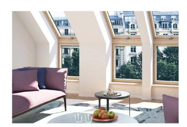
The most eco-friendly roof window on the market today is a triple-glazed and krypton-filled glazing unit with low e-coatings which ensure outstanding heat-insulating performance, and an Uw parameter of 0.99 W/m<sup>2</sup>K. Krypton gas-filled pane construction conducts heat by 46% less than the most frequently used alternative Argon.
